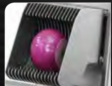
Unique quick change pusher/hopper design keeps fingers completely away from blades and hold product in perfect slicing position
