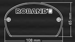
Dimensions for fabricator quartz heating and infra-red heating assemblies (HUQ & HUE)
